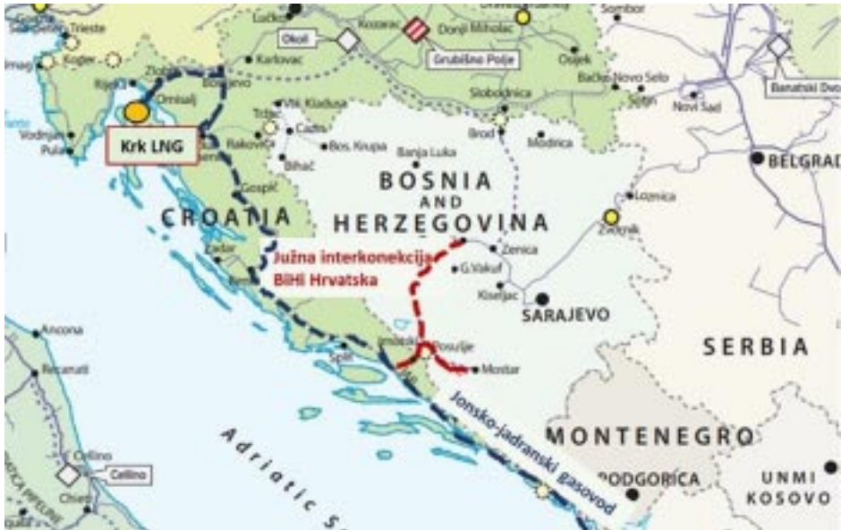
Figure 23 A more detailed overview of the existing and planned gas pipelines in BiH with an emphasis on the Southern Interconnection
