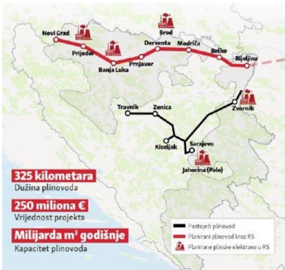
Figure 22 Gas pipeline to Banja Luka and Croatia “New Eastern Interconnection” from Turkish Stream. 32
